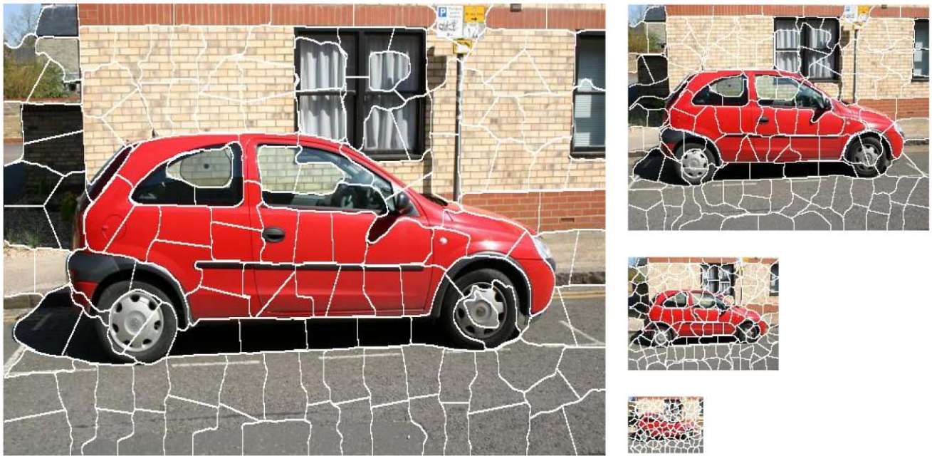
Fig. 5 An example demonstrating that approximately the same number of superpixels (100) can be used at different resolutions with negligible differences in terms of capturing the salient details in the image.
