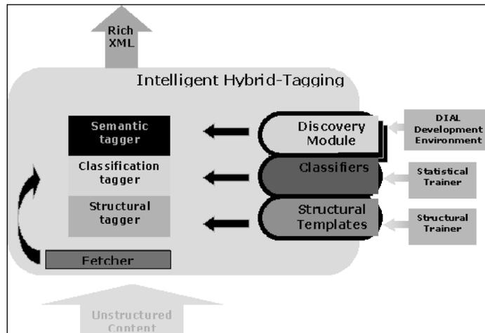
FIG. 9. Architecture of the hybrid tagging system.
