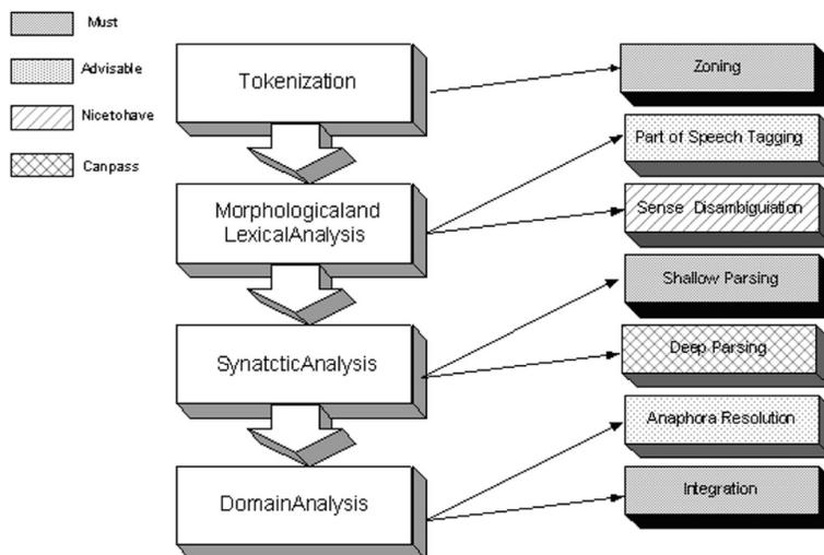
FIG. 5. Architecture of a typical information extraction system.
